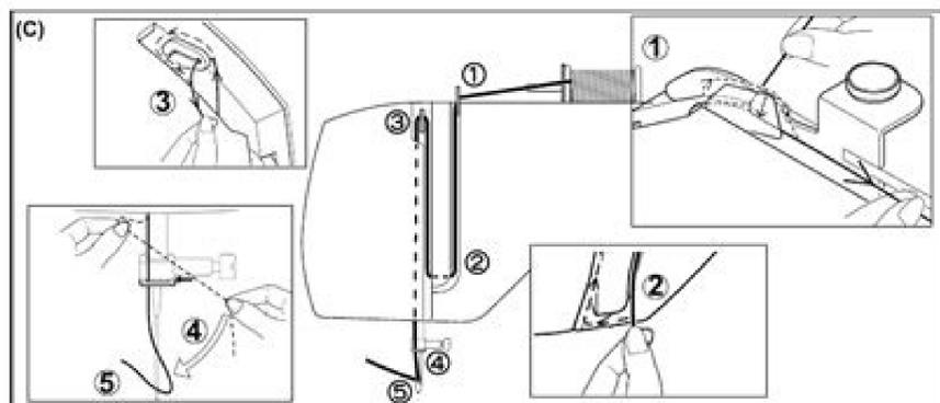
C. Thread the machine with your left hand while firmly gripping the thread with your right hand in the following order as illustrated.
